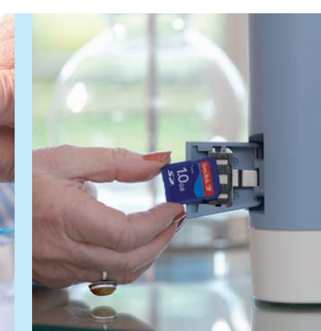
1GB SD card to store up to 1 year of ventilation data.
