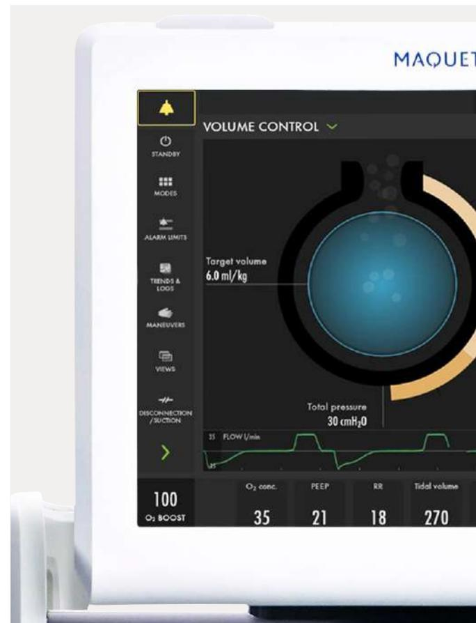
Servo Compass visualizes the volume and pressure of each breath in relation to set targets.
